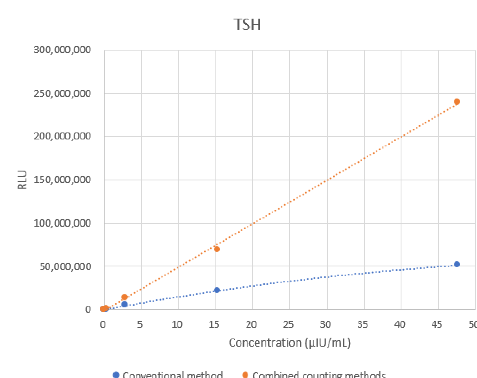
Figure 8 Access TSH (3 rd IS) assay comparing conventional (photon-counting only) vs. new combined counting method
