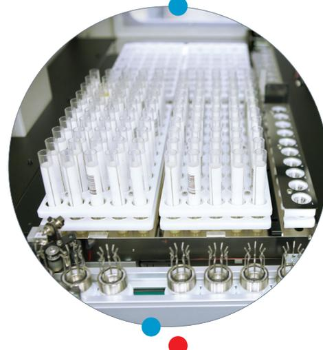
Featuring a combined 200-tube inlet/outlet as well as a 10-position priority-load area, Power Link delivers automated specimen processing power and flexibility to meet your laboratory workload challenges.
