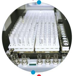
Featuring a combined 200-tube inlet/outlet as well as a 10-position priority-load area, Power Link delivers automated specimen processing power and flexibility to meet your laboratory workload challenges.
