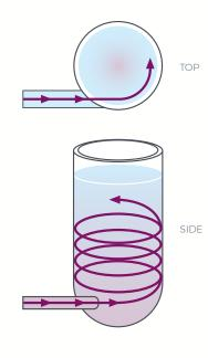
Figure 1. Tangential Mixing
