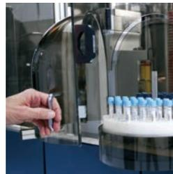
The broth enrichment/Kirby-Bauer inoculation module provides automatic inoculation of enrichment broth and Kirby-Bauer plates with no labeling required.
