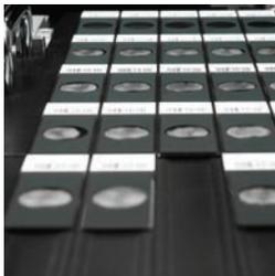
The Gram SlidePrep module reduces staff time by automating Gram slide preparation and permanently printing barcoded patient and specimen information on the slide.
