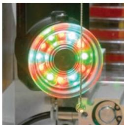
The image analysis verification system confirms accuracy and integrity of the loop as well as the presence of inoculum.
