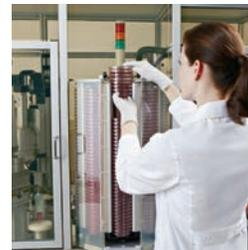
The media carousel consists of nine silos and holds up to 378 plates of any manufacturer's standard media to accommodate most plating protocols.
