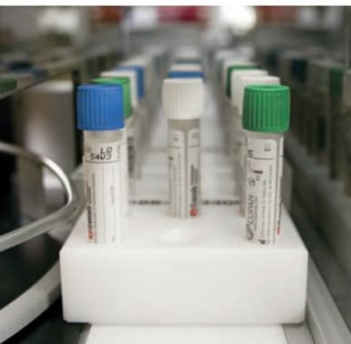
The specimen incoming conveyor system allows continuous feeding of any sample type. Use of pallets means specimen batching is not necessary.
