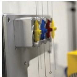
The loop and tool change station allows for longer walk-away time and less user intervention by automatically selecting the appropriate inoculation tool (available in 1, 10 and 30  $\mu$ L loop sizes).
