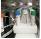
The specimen incoming conveyor system allows continuous feeding of any sample type. No batching is necessary when using pallets.
