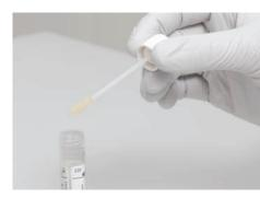
ESwab's unique cap design allows the applicator stick to securely attach to the cap so the swab can be conveniently removed and manipulated by using the cap as a handle.
